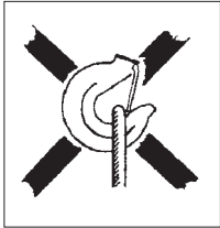
Fig 2a The sling is applying load to the hook tip.
