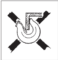
Fig 2d Hook tip subject to additional bending stress.
