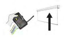
5. Push the up button again. Make the screen go up till the upper stop position. Once there, the motor will stop automatically; Do not leave the button, but keep the button pushed.
